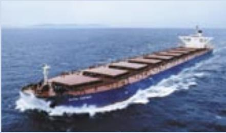
**Bulk Carriers** are the work horses of the fleet, transporting raw materials such as iron ore, coal and foodstuffs, identifiable by the hatches raised above deck level which cover the large cargo holds. **The largest bulk carriers can transport up to 200,000 tonnes of grain, enough to feed half a million people for a year.**
