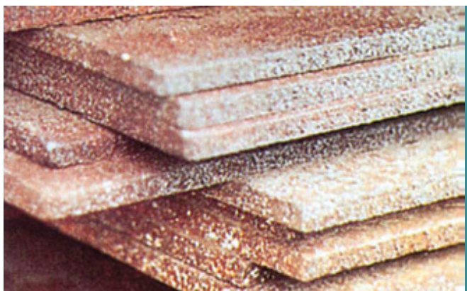
Plates - Surface-condition clause: rust with pitting.
