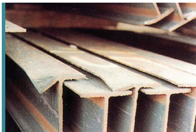
Nest of beams - Mechanical-damage clause (left hand beam): flange bent in one position at end.
