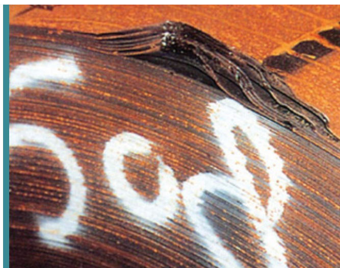
Coil damaged by forklift - Mechanical-damage clause: edges buckled at outer circumference where handling gear marked. Affects six windings.
