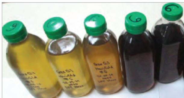
Marine Gas Oil (MGO) on left and Marine Diesel Oil (MDO) on right
