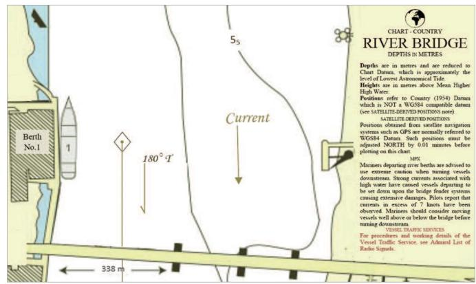
The International Convention for the Safety of Life at Sea (SOLAS), chapter V, regulation 34, requires that masters shall, prior to proceeding to sea, plan the passage from berth to berth. For pilotage the plan should at least give a basic indication of preferred intent. But in practice what does that mean for masters faced with getting their ships away from the berth and safely on passage? This is a question North wishes to put to Signals readers by asking for responses to a case study.
