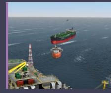
Offshore loading operations from Floating Production Storage Offloading vessels (FPSOs) in Brazil are usually carried out by dedicated dynamically positioned (DP) shuttle tankers. The shuttle tanker's bow loading system connects to the FPSO's offload hose and its dynamic positioning system is used to position the shuttle tanker during the loading operation.
