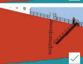
If the distance from waterline to the boarding point is more than 9 metres then a combination arrangement must be used - the accommodation ladder combined with a proper pilot ladder. Check the rules for rigging distances.
