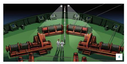
Mooring stations should be adequately lit and kept free from obstructions which could hinder the safe movement of personnel or obstruct lines of sight between members of the mooring party. Decks should be clean, free from oil or grease and coated with anti-slip paint. Is the mooring station design adequate to ensure the safety of personnel e.g. is the winch operator in a snap-back zone?
