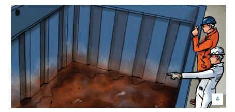
The master should observe the start of loading and look and listen for signs of splattering (muddy splashing) of the cargo on tank tops and bulkheads. This is an indication that the cargo may be in a fluid condition.
