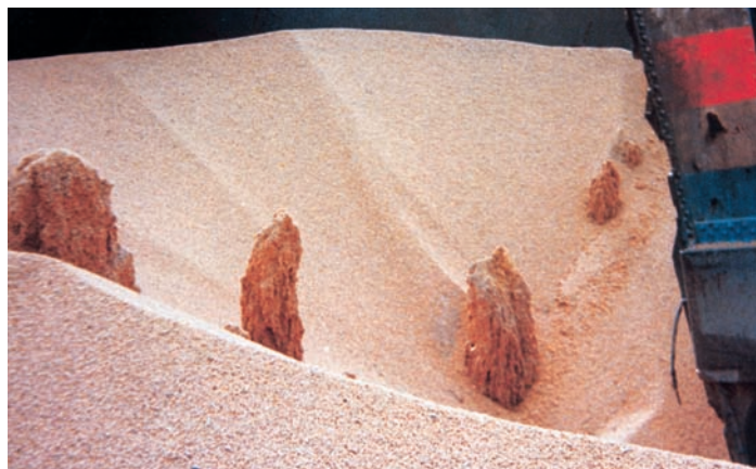
Fig. 1 Damage to cargo caused by water ingress resulting from poor hatch cover condition
