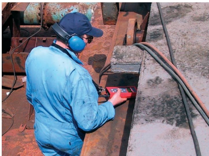
Fig. 34. Conduct of an ultrasonic leak-detection test
