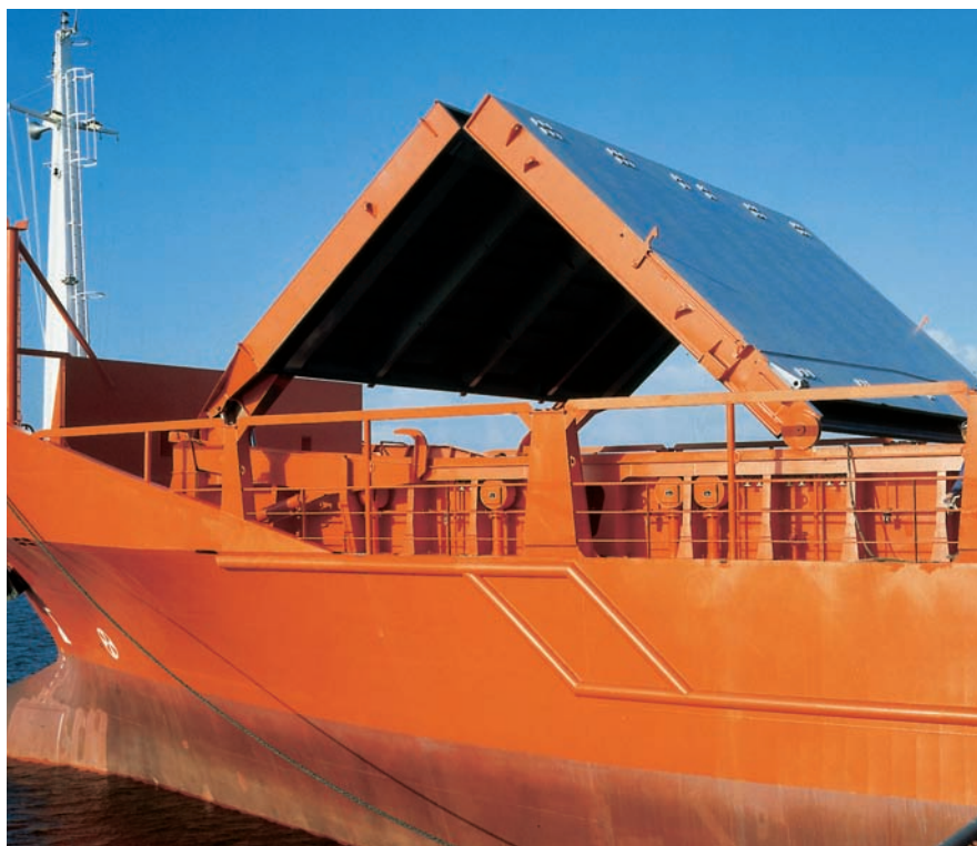
Fig. 2. Hydraulic folding pair of hatch covers 'peaked' during opening
