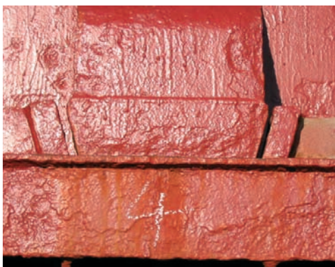
Fig. 22. Hatch cover locator, showing clearances
