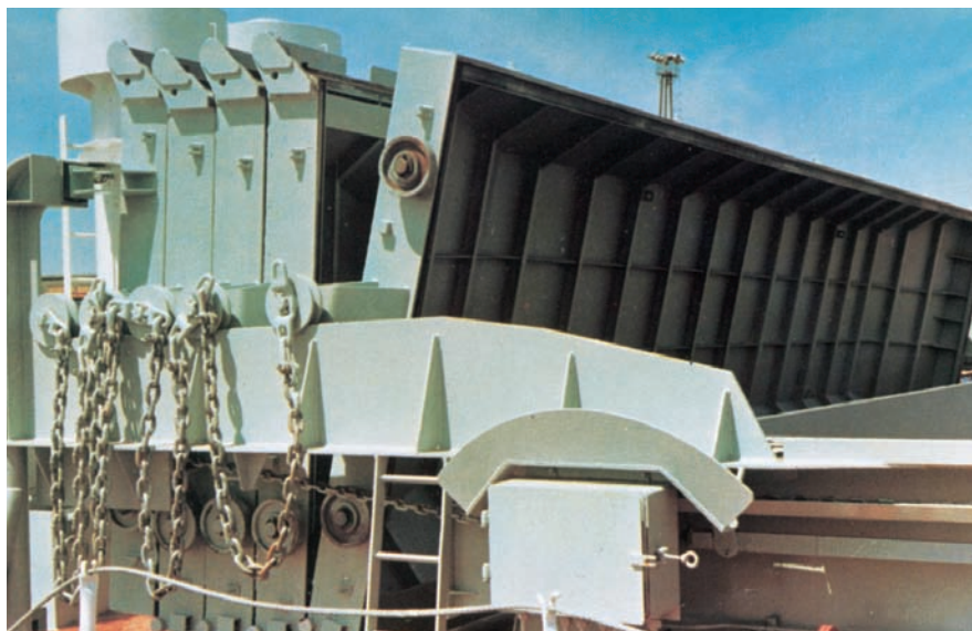
Fig. 7. Single-pull hatch covers with long-chain drive operation
