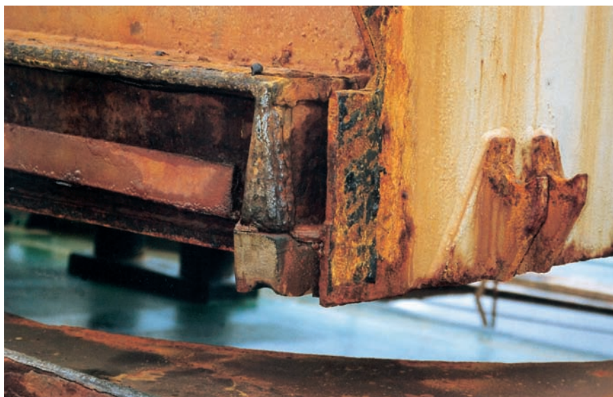
Fig. 20. Cross-joint of a corroded hatch cover showing the compression bar with drain channel below it and drain hole in the side plate
