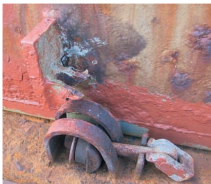
Fig. 29. Cleat and cleat snug in poor condition
