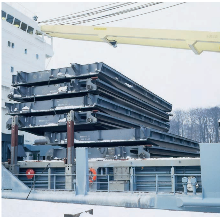
Fig. 12. Typical multi-stacking hatch covers showing four panels stacked and two panels rolling beneath
