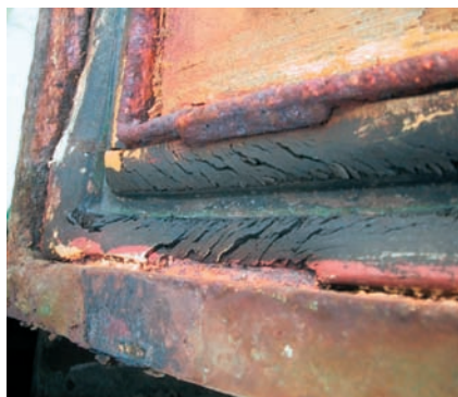
Fig. 24. Seal in very poor condition, showing permanent set
