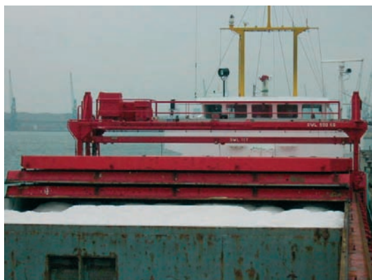
Fig. 13. Gantry crane operation of hatch covers
