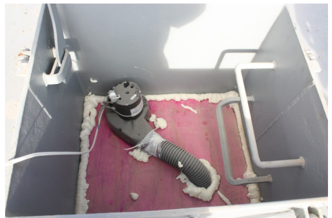
Recirculation fan positioned in hold access trunking
