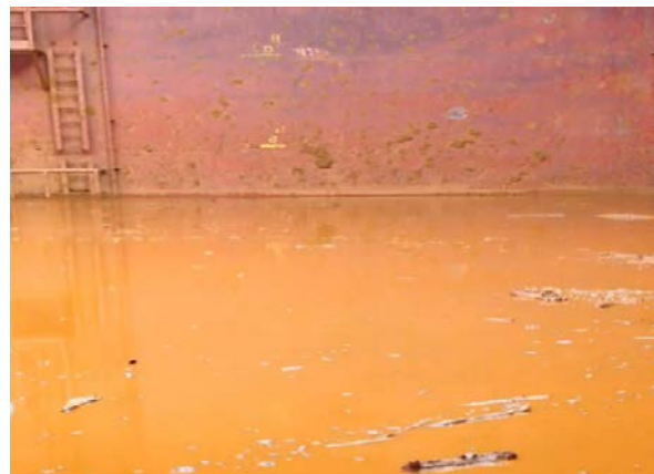
Figure 4 - Liquefied cargo (Photo: Roxburgh Environmental Ltd)
