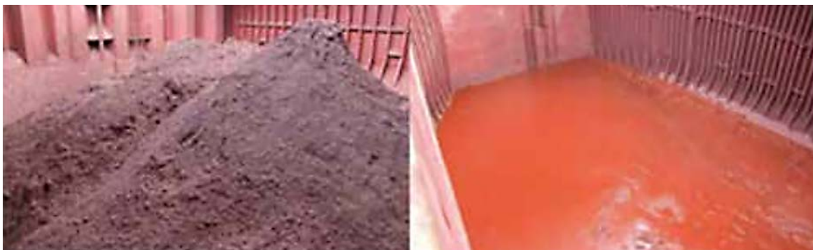
Figure 10 - Iron ore fines before and after liquefaction (Photo: Gard)
