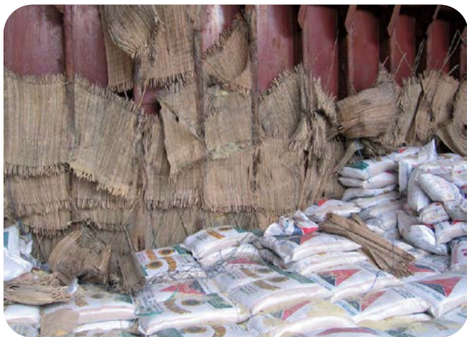
Figure 5: Bamboo and bamboo matting used for dunnage can be too thin and unsuitable
