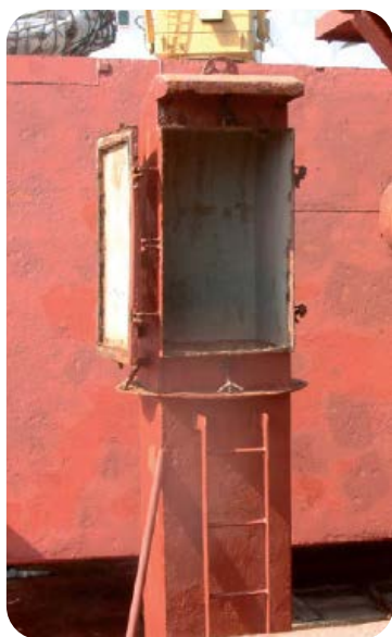
Figure 9: Some ventilation heads can expose the hold to ships spray depending on their design, position and height on the vessels deck.
