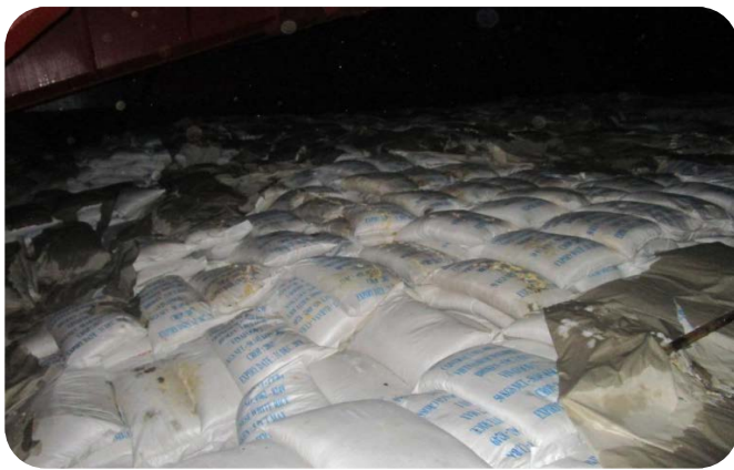
Figure 1: Bagged rice cargo covered in damp Kraft paper.
