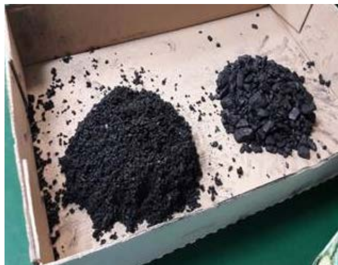
Figure 4: Coal sample after separation approximately 60% fine particles and 40% lumps.
