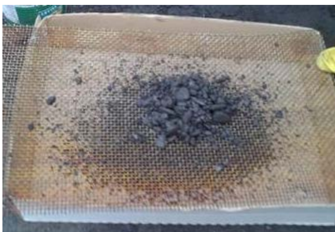
Figure 3: Separating fine particles and lumps of coal
