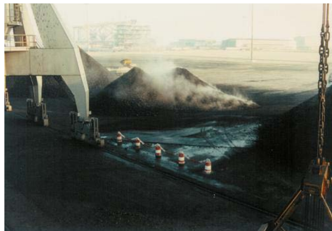
Figure 7: Steam rising from heating coal
