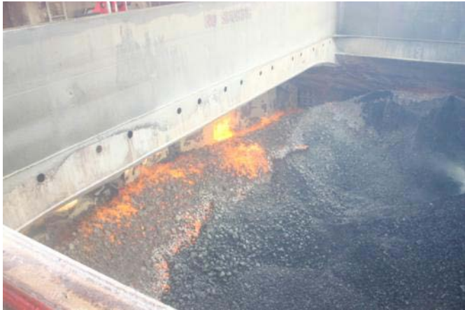
Figure 8: Coal on fire in a ship's hold
