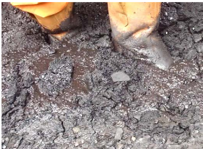
Figure 6: Damp coal underneath a dry crust
