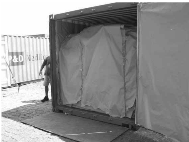
Figure 2: Lining paper applied to bagged cargo
