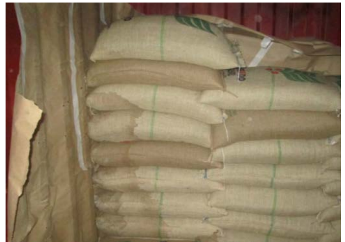
Figure 1: Water stained bagged cargo in a container
