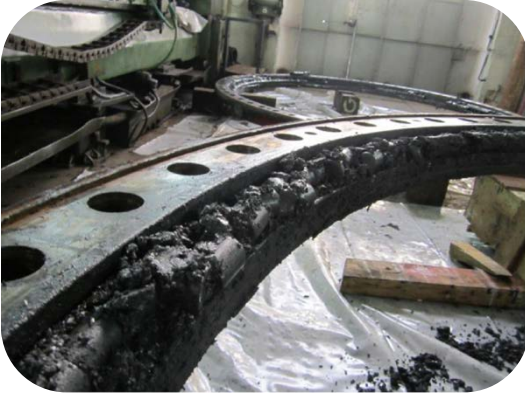
Rollers retaining ring damaged, rollers displaced.
