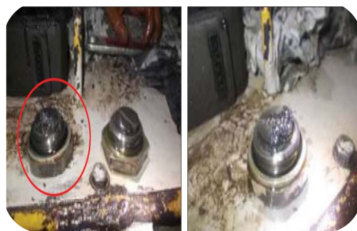
Example of contaminated oil and metal filings on the magnetic drain plug
