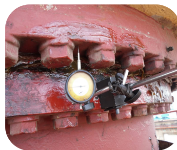
Example of examination with depth gauge and clock gauge
