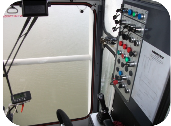
Crane Cab alarm panel
