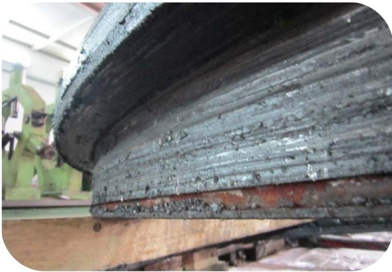
Slewing bearing inner flange with circumferential deep scoring
