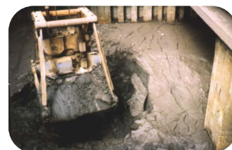
Example of a static load test using water bags and potential dynamic loading situation from a wet bulk cargo
