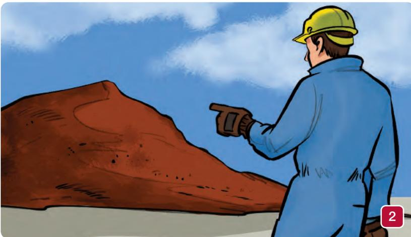
The stockpile should be sighted and/or sampled prior to loading where possible. Photographs of the cargo should be obtained where possible before loading.
