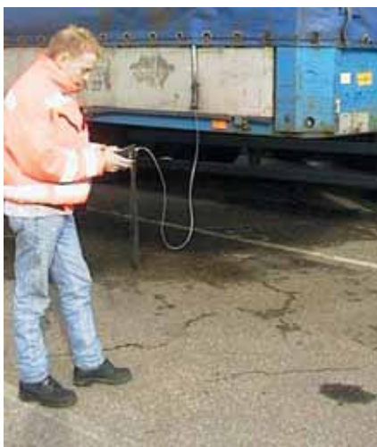
CO2 detector in operation
